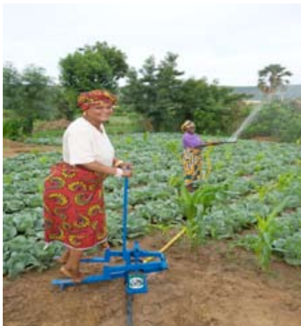
Figure 6. KickStart's Super MoneyMaker Irrigation Pump
